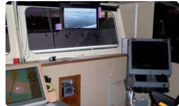
The FLIR Systems Navigator produces a crisp image which is projected on a 20" LCD screen installed on the bridge
