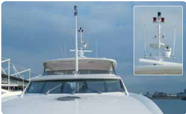
A FLIR Voyager installed on a 34 Metre Yacht
